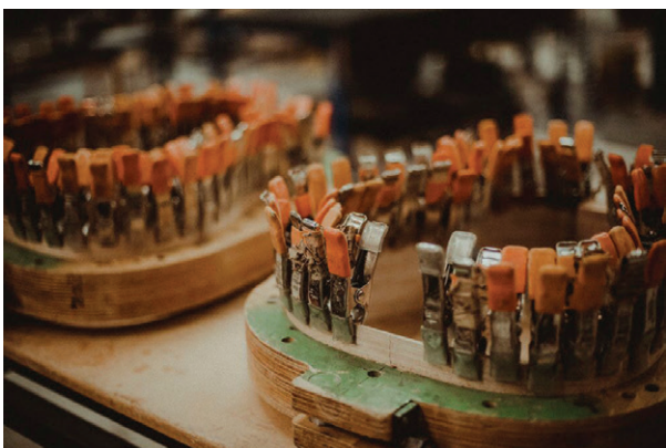
Jigs being used to build the body of a Maton guitar. Image courtesy of Maton guitars.
